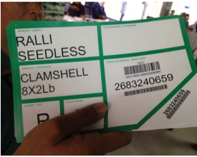
Subsole Pallet label with SAG compliant 10-digit pallet number and 18-digit GSI SSCC
